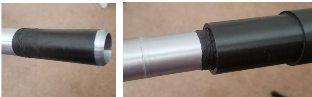
Figure 9: Use of bagpipe waxed thread on the adjustable bocal (Joel Daniel)
