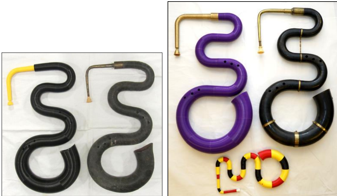
Figure 3: 3D-printed "Anon" serpent and 19th Century original (left). 3D-printed Dittes serpent and original, with ½ sized 3D printed tenor serpent (right)
